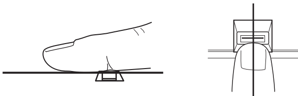
Sample aligning the finger on the sensor
